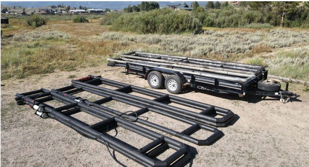
Figure 12. PIT Tag Antennas from first install on trailer (right), on ground (left) new PIT Tag Antennas.
